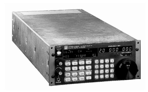
The WJ-8712P is a fully synthesized, general-purpose HF receiver for surveillance and monitoring of RF communications from 5 kHz to 30 MHz with 1-Hz tuning resolution. The unit is packaged in a 3.5 x 8.25 x 20 inch (8.89 x 20.96 x 50.80 cm) half-rack enclosure, and utilizes the same RF and Digital printed circuit boards as the WJ-8711A. By combining analog and digital signal processing, the WJ-8712P achieves high performance at low cost.
